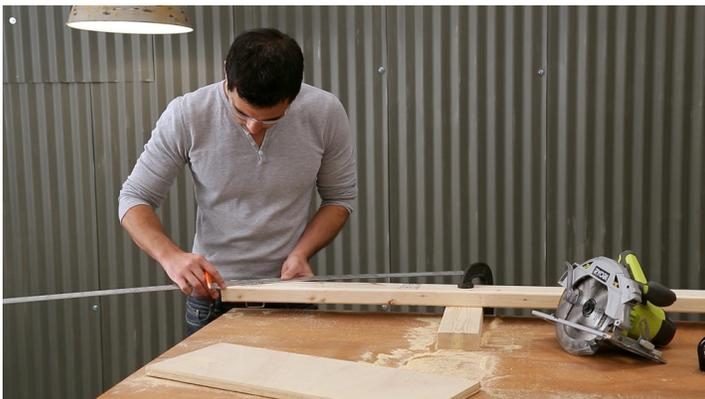
Make the beveled cuts. Clamp down a straight edge so that your cuts across the plywood are straight.
