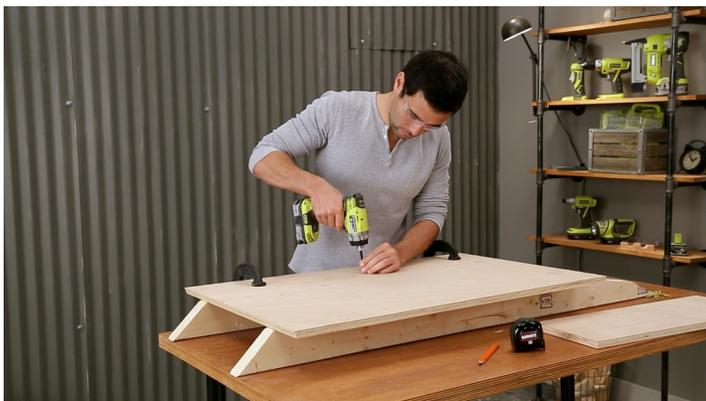
Glue and screw. Use wood glue and 2" screws to fasten the plywood panels to the 2x4s. Clamp the plywood in place or get a friend to help you position the plywood panels while you screw them. Use 2 1/2" screws to connect the 2x4 pieces to each other. Make sure to drive the screws into the plywood until the heads of the screws are level with the surface of the plywood.
