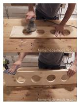
Sand the boards. Pine is a soft wood, so you can hand sand the boards pretty quickly. I used an orbital sander and sanded them with 220 grit paper.
