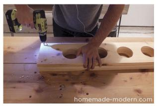
Drill holes for rope. I used a 5/16" drill bit for the 1/4" rope. It's important to have a tight fit for the rope so that the zip ties create a stopper to keep the boards from sliding.
