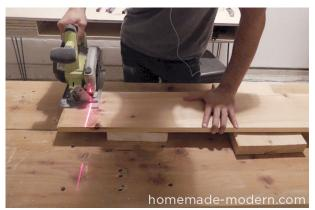
Cut the boards. Once you have established the hole locations, you can trim the boards to the desired length with a circular saw. If you lay out the boards in advance, you can have the boards cut for you at Home Depot. I purchased 6' boards and cut them in half.
