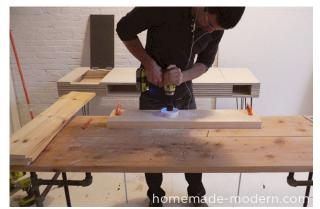
Cut holes for pots. Hole saws can be a bit tricky to handle. The larger diameters can generate a lot of friction with wood so it's important to properly secure the boards and have a firm grip on the drill. I clamped the boards two at a time to a work table. Set your drill to the drilling mode at the highest speed and use both hands. The saw will occasionally freeze up and bind against the wood, so be patient and try and keep the drill perpendicular to the board.
