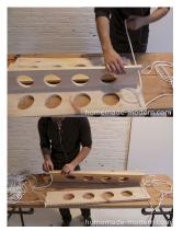
String the boards.. Thread the rope through the holes and tie a knot at the bottom.
