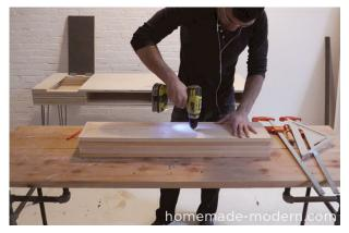
Drill pilot holes. The key to this project is making sure the holes are aligned. Rather than marking each board, I simply marked one and drilled small pilot holes through the entire stack of boards. These small holes will serve as guides for the hole saw.
