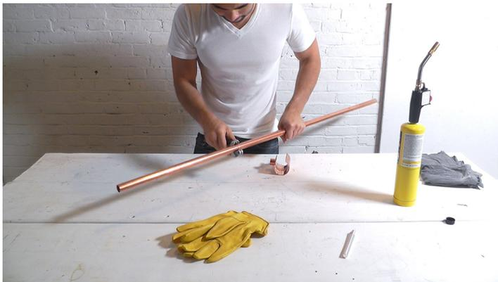
Cut the Copper Pipe I used my RIDGID Tube Cutter to cut the copper pipe.
