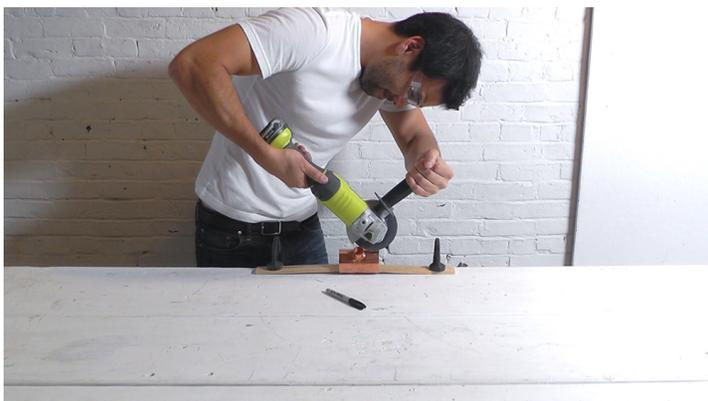
Cut the Copper T-Fitting I used my angle grinder with a metal cutting blade to cut along the lines that I drew on the T-fitting. I cut a groove along the line at first and then went back and cut through it with a second pass.
