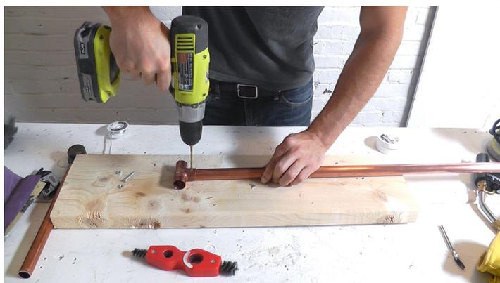
Attach the 3/4" T I could have soldered the 3/4" T to the other side of the pipe, but I thought I would try a mechanical connection instead. I inserted the pipe into the fitting and then drilled a hole through both the T-fitting and the pipe. I pushed a bolt through the holes and fastened it with a nut.
