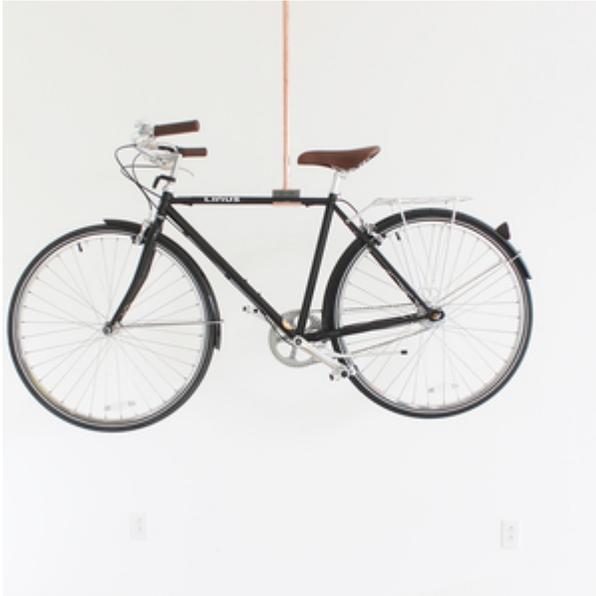
This Copper Bike Rack is made from copper pipe fittings and a small piece of felt. I used an angle grinder to make two cuts along a 2" to 3/4" reducer T fitting. I soldered the cut T-fitting to a length of 3/4" copper pipe and then used a nut and bolt to connect the other end of the pipe to a 3/4" T-fitting.
