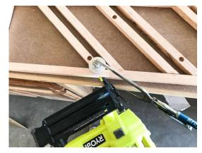
For the ends that attach to the outside frame, use 1 1/4" brad nails, driven in at a slight angle along with wood glue.
