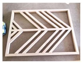
For the arrows, cut 2 pieces at 3" long with perpendicular 45 degree angles. Cut 2 pieces at 6" long with 45 degree perpendicular angles. Cut 8 pieces at 11 3/16" long with 45 degree parallel angles.
