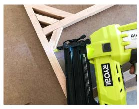
Once the holes are drilled, begin assembling the arrows. Starting with the smallest pieces, use 3/4" brad nails and wood glue to attach to the frame. 3/4" brad nails will be used on all pieces attaching to the center dowel.
