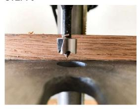
Drill a 5/8" deep hole with a 1/2" drill bit. On a drill press, set the bottom plate of the drill to the proper depth. If using a drill, mark the bit with tape 5/8" up from the tip. Drill holes where marked on the dowels.
