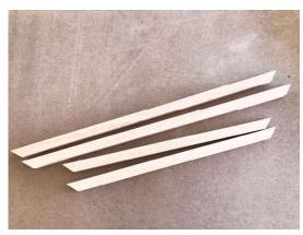
Cut the 3/4" square dowels to size. With 45 degree perpendicular angles, cut two at 24" and two at 18".
