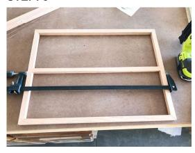
Measure and cut to size the center dowel (approx. 22 1/2"). Add glue to each end and center it in the frame. Attach with 1 1/4" brad nails.
