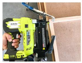
Assemble the frame. Glue and clamp the pieces together. Attach with 1 1/4" brad nails.
