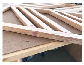
Set nails as needed. Fill nail holes with wood filler and sand with 220 grit sandpaper.
