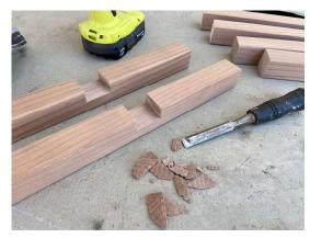
STEP 2: Align your two 13 1/8" pieces and mark out a section of approx 1.5" in the center to be cut. From center this will be approx. .75" in each direction.
