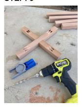
STEP 3: Now set the depth of your circular saw at just .75".... or 3/4". Using the saw make several cuts in parallel on the 'marked' sections on your 13 1/8" pieces. (This is from step 1)
