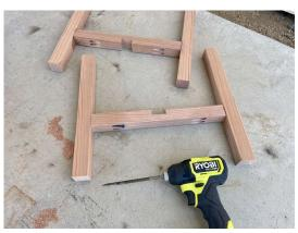
STEP 4: Knock out the thin material in between these cuts to create a half lap joint. This notched area should not be deeper than 1/2 the material thickness.
