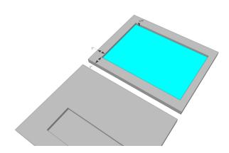
Using your router set to the same depth, cut out a space on the upper board (this will be where the chalkboard resides) according to the dimensions on the picture.
