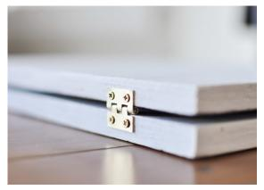
Attach Hinges so that when the "laptop" is open the hinges stop when the upper board is in the correct position for use.
