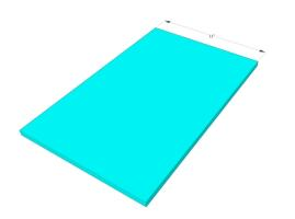
Using a table saw, rip your 1/2" sheet of plywood down to 11".
