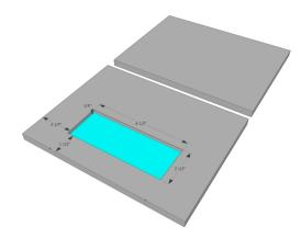
Use your router, set to 1/4" depth, cut out a space according to the dimensions on the picture.
