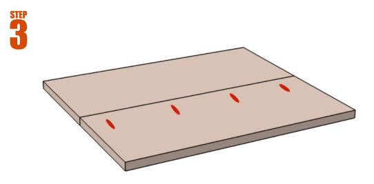
Drill pocket holes and assemble top with 1–1/4" pocket screws.
