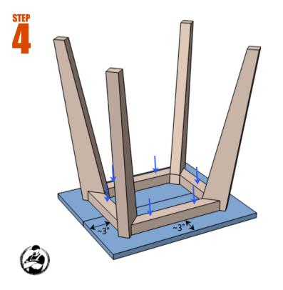
Center base on bottom of top and attach with **2" wood screws**.
