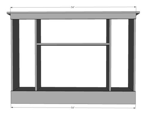
Step 2: Attach header and footer to front.
