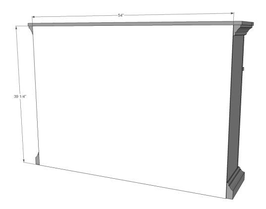
Step 7: Back is attached with  $\mbox{\%}''$  brad nails and glue to all carcass boards.
