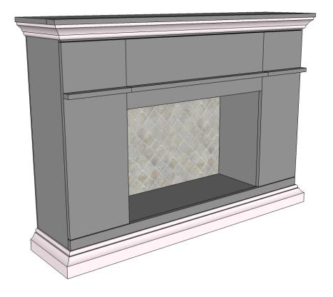
Step 6: Cut moulding to fit and attach with  $1^{\prime\prime}$  brad nails and glue.
