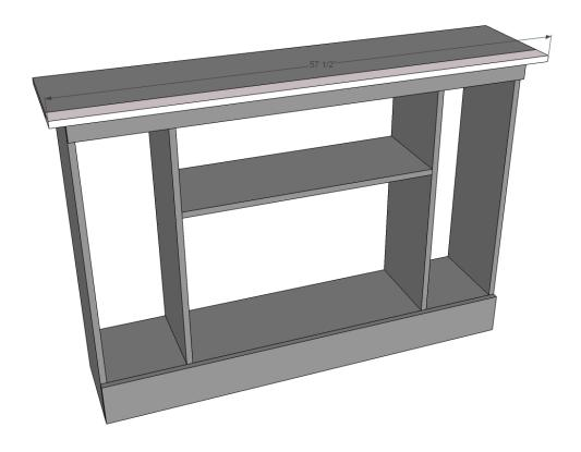
Step 3: Attach front top header piece to top, using  $\frac{3}{4}$ " pocket holes and 1-1/4" pocket hole screws and glue. Also glue and nail to bottom header piece with 1-1/4" brad nails.
