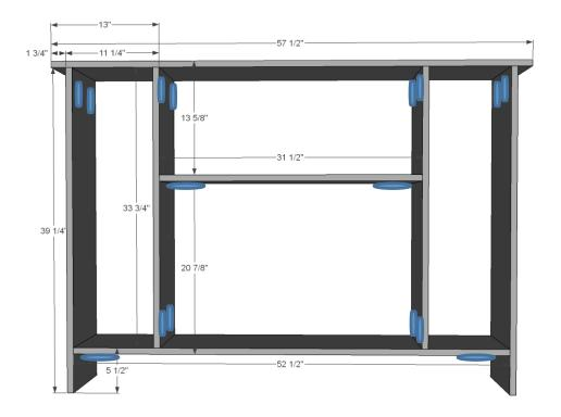
Step 1: Build carcass with  $\frac{3}{4}$ " pocket holes and 1-1/4" pocket hole screws and glue.
