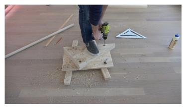
4. Drill holes in the triangles I tried a 1.25" diameter wood dowel for the bar but it was too weak.  $\frac{3}{4}$ " diameter steel pipe works well with but I prefer wood. I found a 1.5" diameter maple dowel 36" long and used that for my chin up bar. I drilled 1" diameter holes to accommodate  $\frac{1}{2}$ " iron pipes 9" long on the longest side of the triangle.
