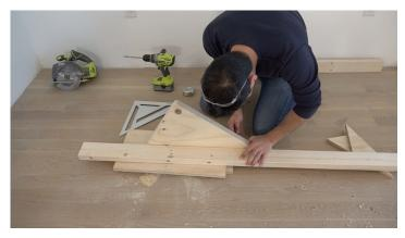
6. Drill matching holes in the 2x4s I used the triangles to mark hole locations on the sides of the 2x4s. I then drilled 1" diameter holes in the 2x4s. The holes should be right along the edge and come close to busting through the side of the 2x4 leaving  $\frac{1}{2}$ " of wood on the other side.
