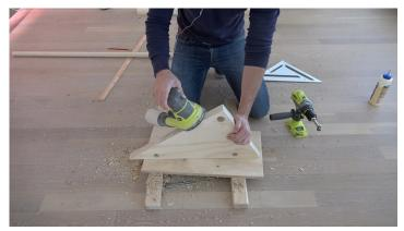
5. Sand the triangles I used my orbital sander to sand down the edges for the triangles.
